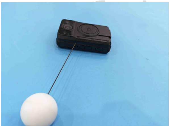
The test stick cannot enter the gap of the sample
